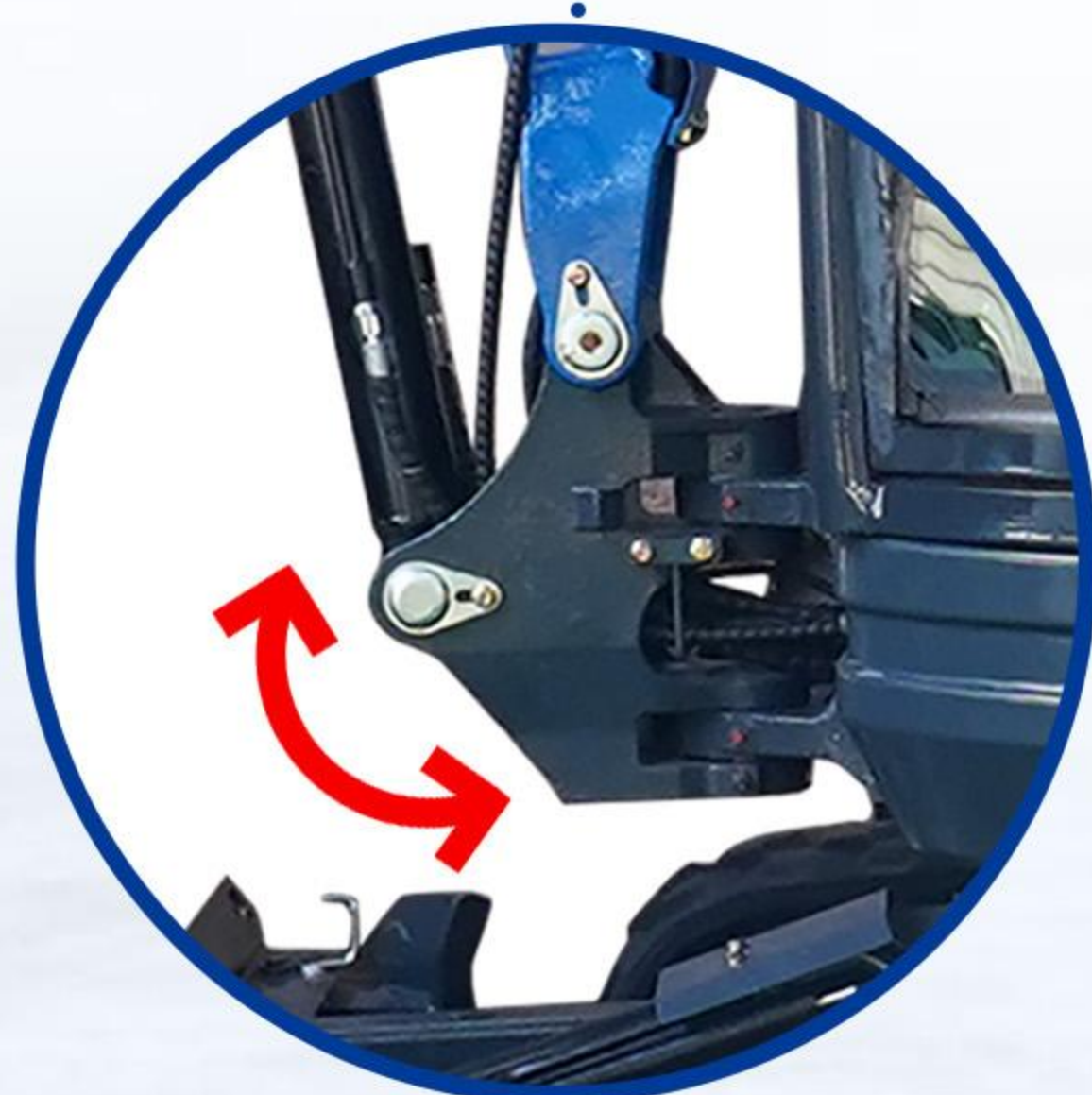
One-piece casting boom bracket + big arm side swing
