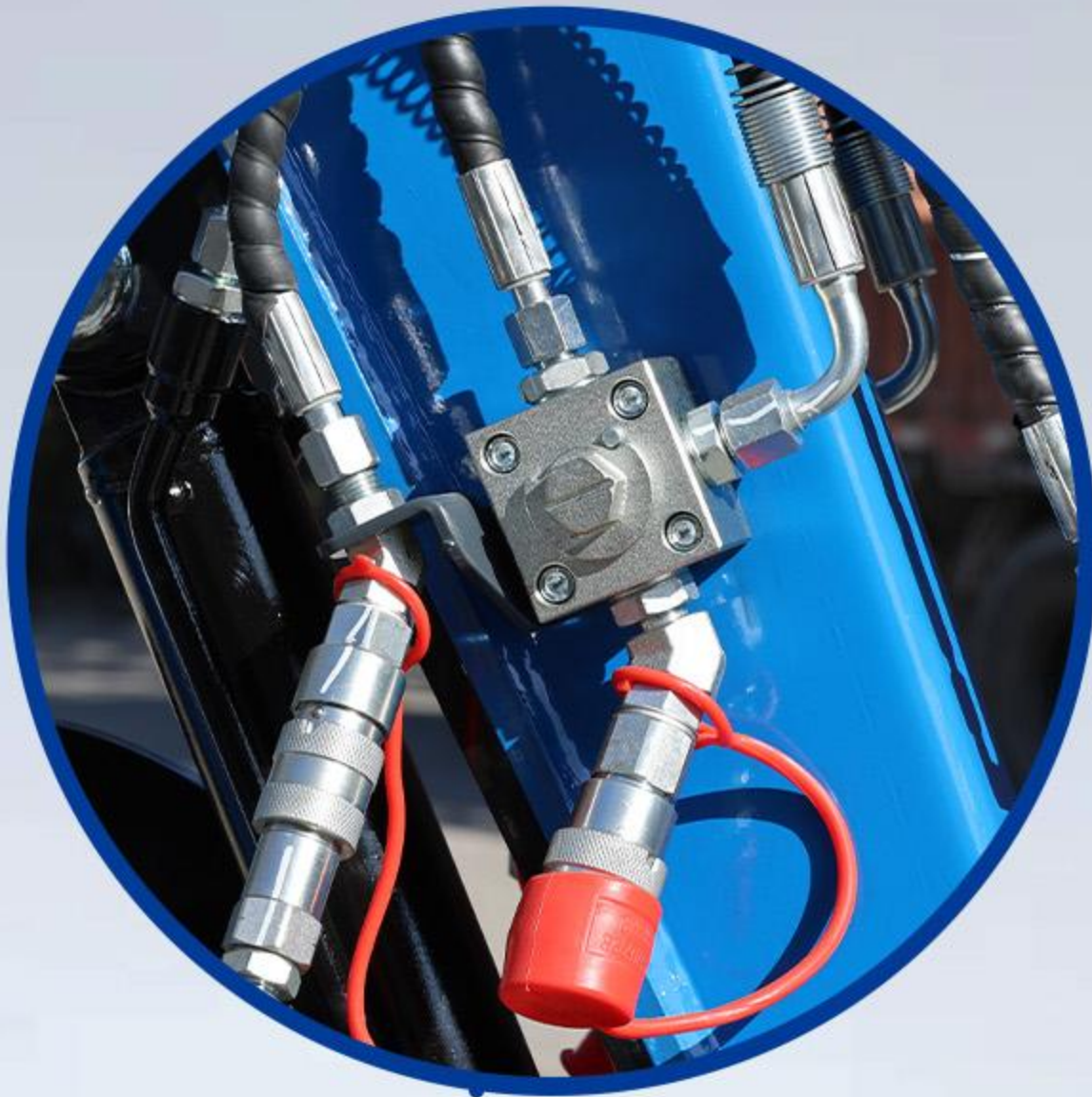
Four pipelines + Globe valve
